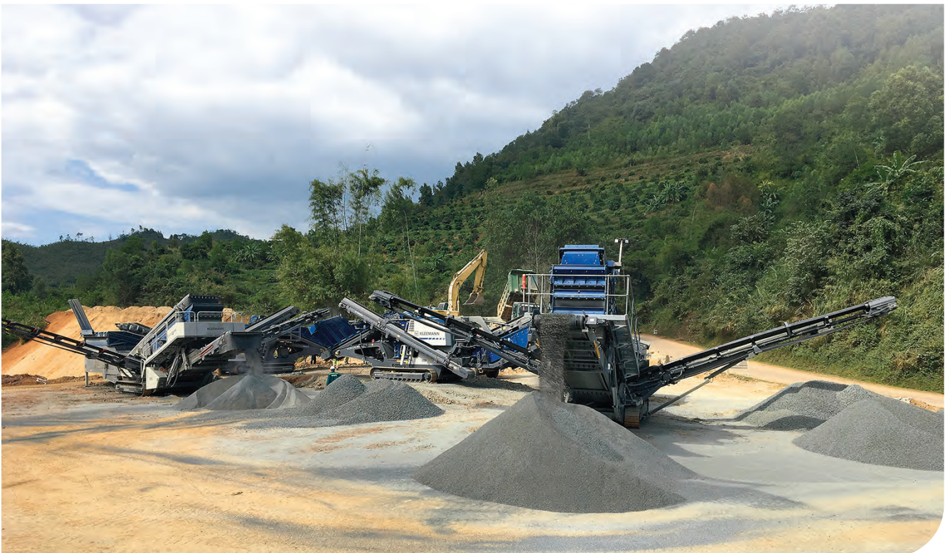
Line coupling enables the Kleemann crushing and screening plants to control their optimum performance automatically, and also minimise the downtimes associated with material blockages including the manual work involved in removing them.
