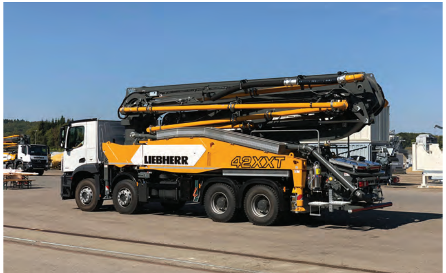
Liebherr 42 M5 XXT truck-mounted concrete pump (above), and the Powerbloc hydraulic unit (left) that is designed exclusively to power concrete pumps.
