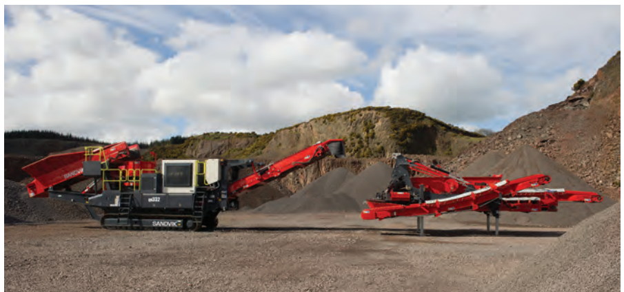
The Sandvik UJ440i mobile jaw crusher is designed for trouble-free operation, thanks to its onboard integrated 'intelligence' system.
