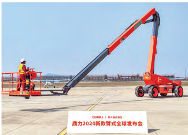
ABOVE: The new EAB28ERT electric articulating boom lift from Dingli has a 28.1-m working height and 230 kg maximum load capacity.
