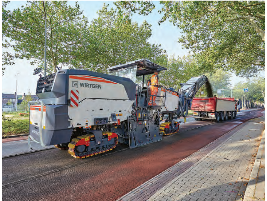
ABOVE AND BELOW: The new Wirtgen W 220 Fi and W 250 Fi large cold milling machines serve a wide range of applications at a maximum milling depth of 350 mm. Various drive concepts are available to ensure excellent milling performance, including a two-speed Dual Shift powershift transmission for the W 220 Fi (above) and an Active Dual Power dual engine drive for the W 250 Fi (below).
