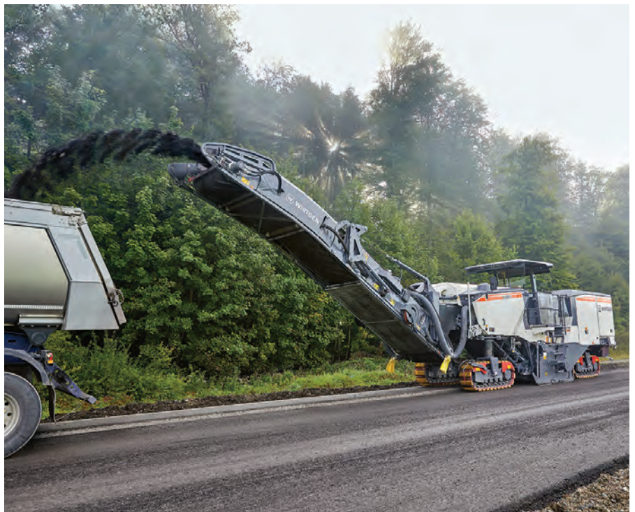
ABOVE AND BELOW: The new Wirtgen W 220 Fi and W 250 Fi large cold milling machines serve a wide range of applications at a maximum milling depth of 350 mm. Various drive concepts are available to ensure excellent milling performance, including a two-speed Dual Shift powershift transmission for the W 220 Fi (above) and an Active Dual Power dual engine drive for the W 250 Fi (below).
