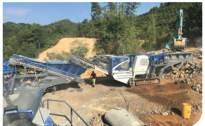
ABOVE (LEFT AND RIGHT): The interlinked Kleemann plant combination, consisting of three crushing and two screening plants, were used to process the basalt for the surface course.
