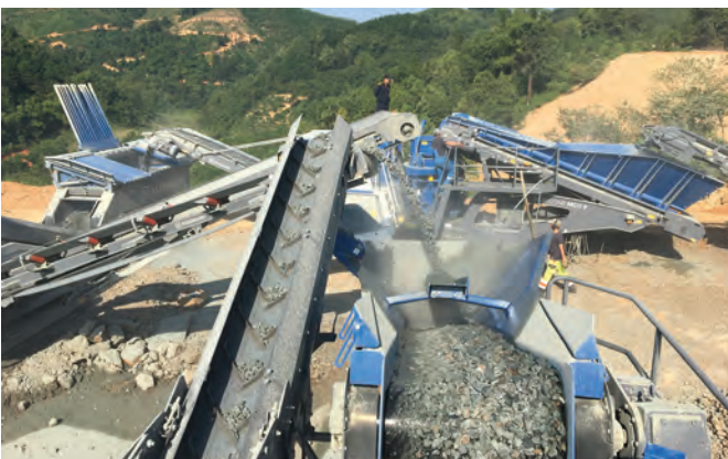
ABOVE (LEFT AND RIGHT): The interlinked Kleemann plant combination, consisting of three crushing and two screening plants, were used to process the basalt for the surface course.
