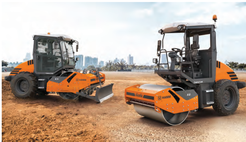
The Hamm H 5i and H 7i H CompactLine compactors feature a compact design and high versatility, with a climbing ability of up to 60%. They are designed with three-point articulation for even weight distribution and superior driving stability.
