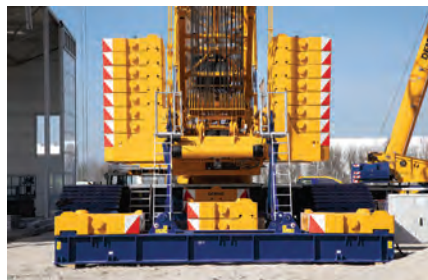
The Superlift Split Tray features quick coupling technology.
