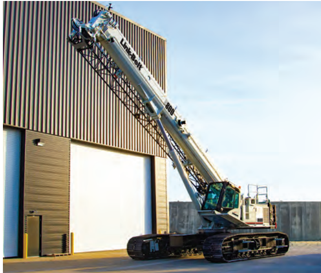
ALL IMAGES: The 75-t TCC-800 telescopic crawler crane is equipped with a four-section 11.8 – 36.5 m full-power boom, which reaches a maximum tip height of 56.2 m (with full boom), as well as Link-Belt's SmartFly pinning system.
