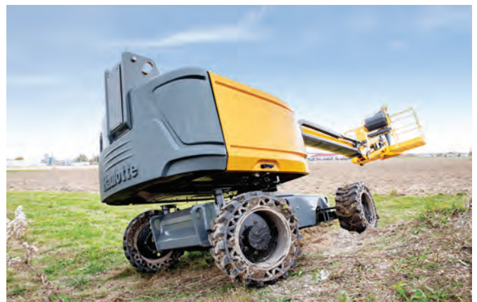
ALL IMAGES: The new Haulotte HT16 RTJ telescopic boom lift (named the HT46 RTJ in the US) has a 16-m working height. The machine is expected to be launched in Europe and Asia Pacific over the next few months.
